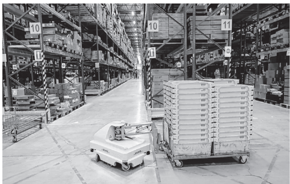
Autonomous forklifts require a signal to direct them as they move pallets.
