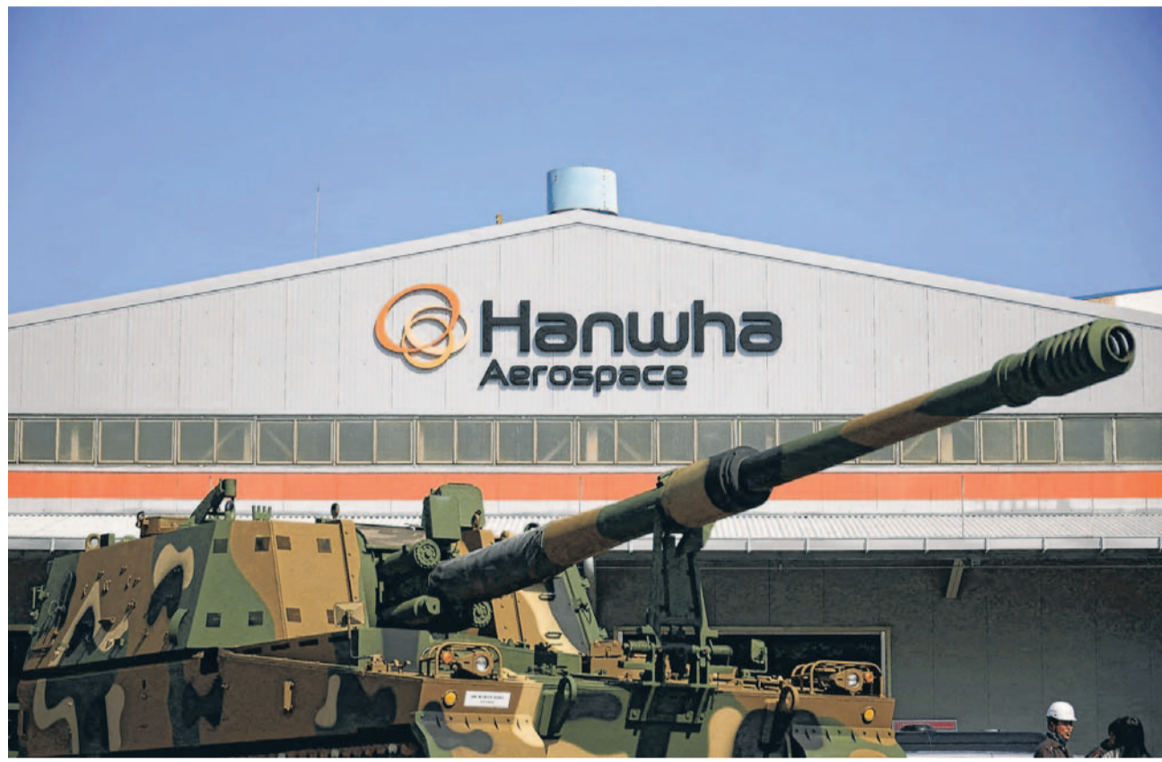
Hanwha Aerospace produces the 155mm K9 self-propelled howitzer, which has become the country’s bestselling weapon.
