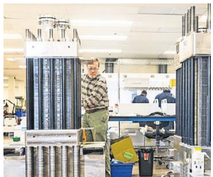
Electrolyser stacks at the Plug Power facility in Concord, Massachusetts
