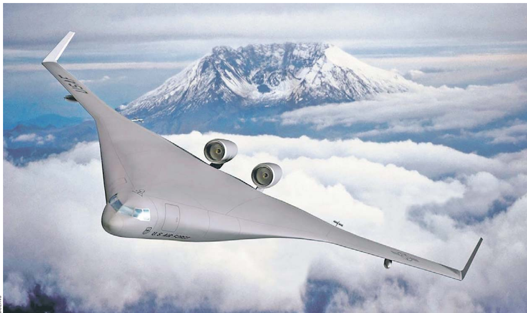
The U.S. envisions a plane with a blended-wing body concept, similar to an Air Force prototype, shown in a 2006 rendering.
