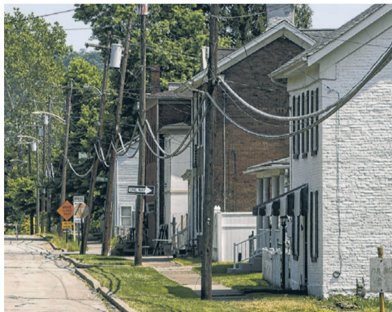
A lead-covered cable, in gray, hangs from poles in Coal Center, Pa.
