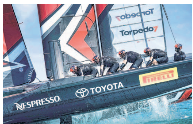
Cyclists helped power the Emirates Team New Zealand yacht’s control systems in 2017.
