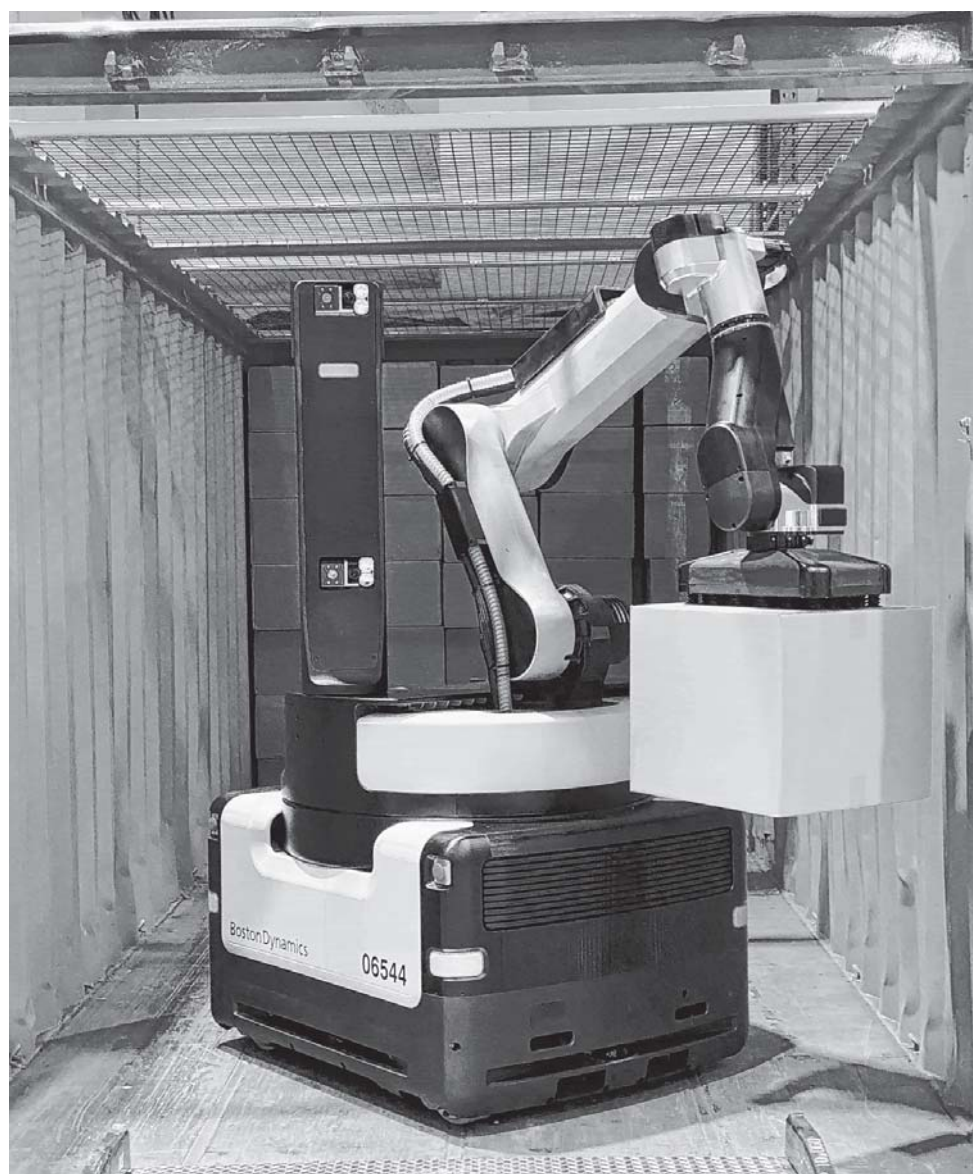
Boston Dynamics' robot Stretch has a 16-hour battery and a single arm with vacuum gripper.
