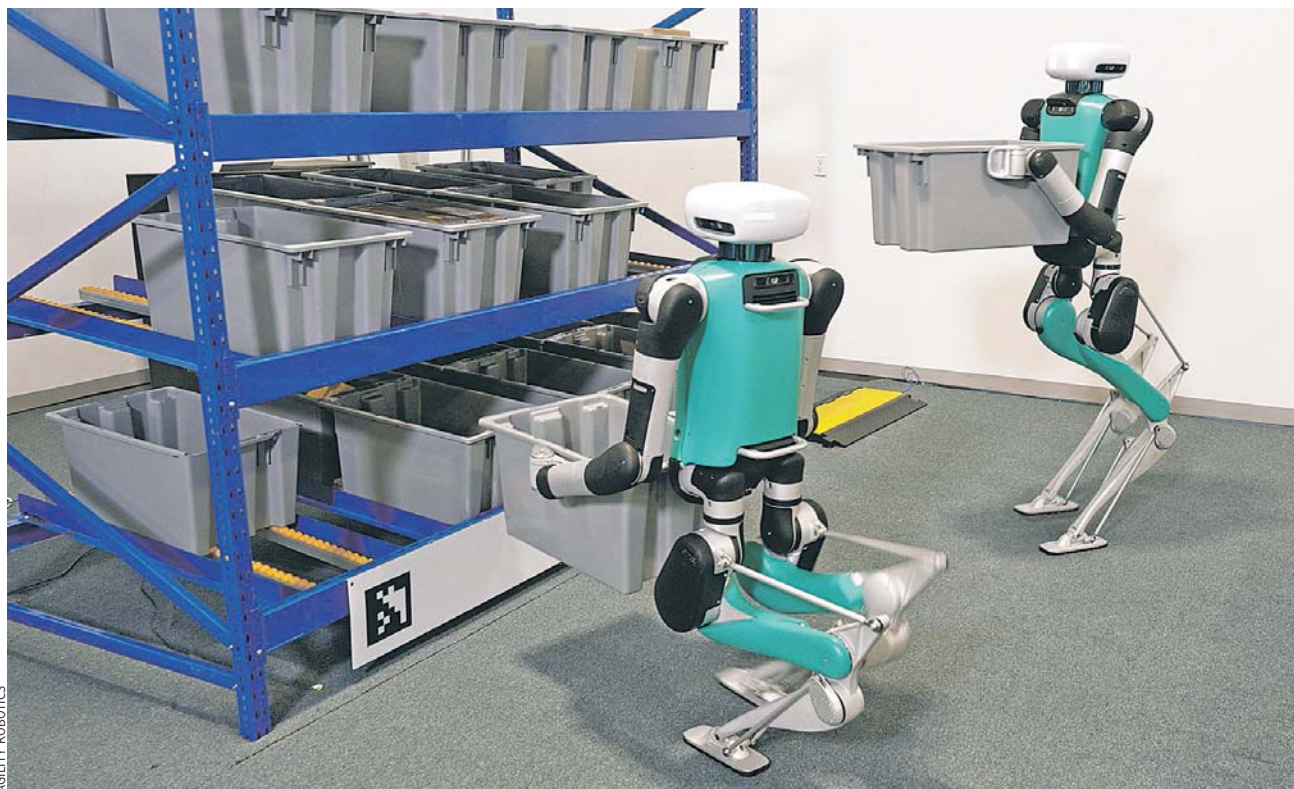
PUMPING IRON: Companies are designing robots that are more closely modeled on human beings, with the ability to walk around distribution centers, and pick up and move boxes. Agility Robotics' Digit robot at its headquarters in Oregon, B4.
