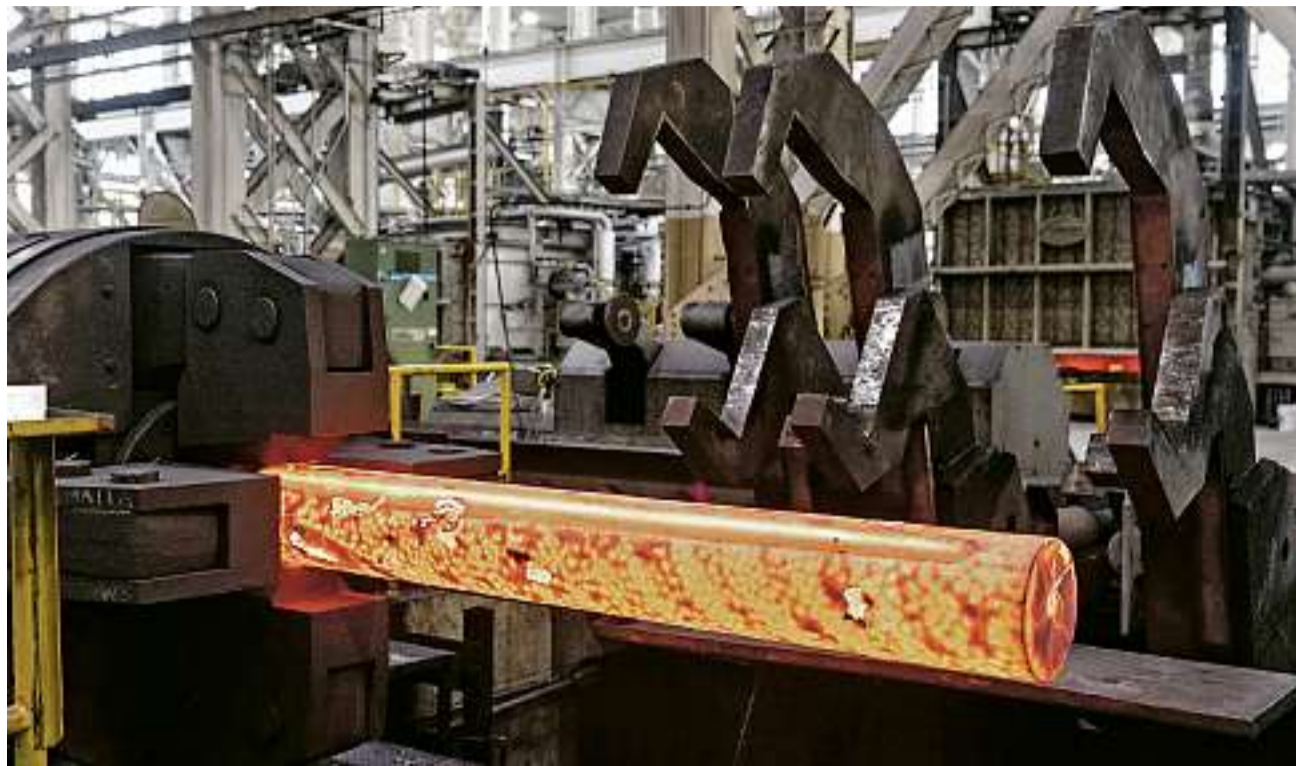
A red-hot steel billet is placed in the rotary forge at the U.S. Army Watervliet Arsenal, which opened during the War of 1812.
