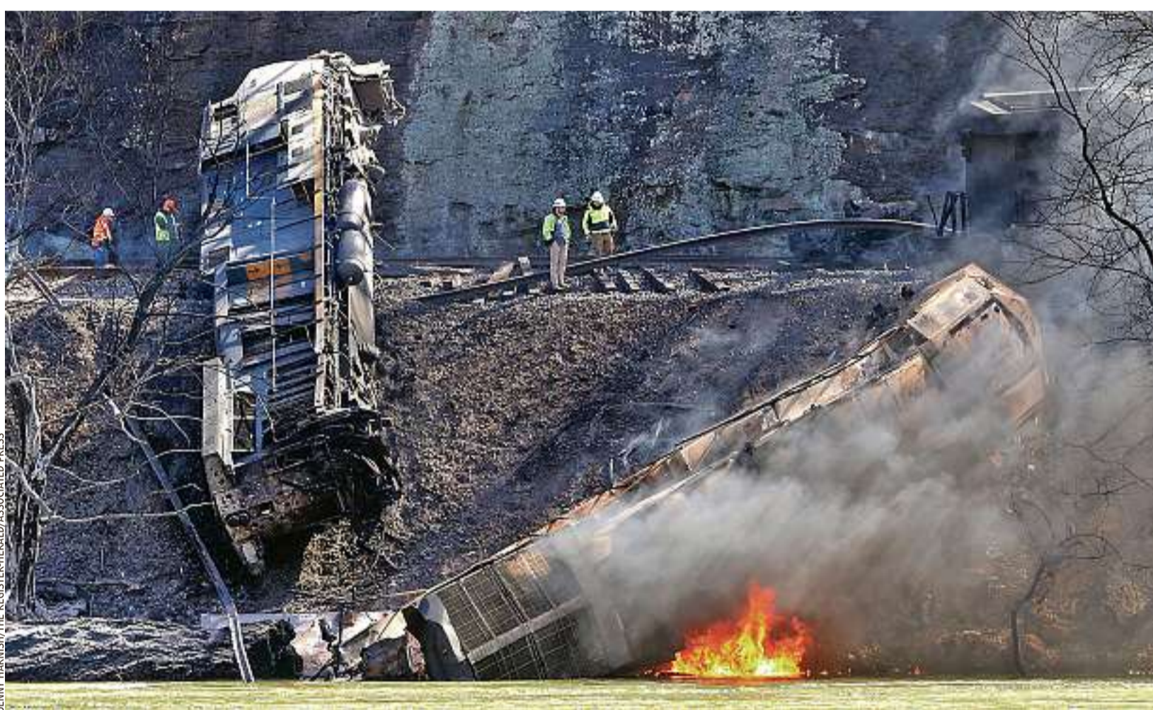
ANOTHER RAIL MISHAP: A rockslide on the tracks caused an empty CSX coal train to derail Wednesday inside the New River Gorge National Park and Preserve in West Virginia.
