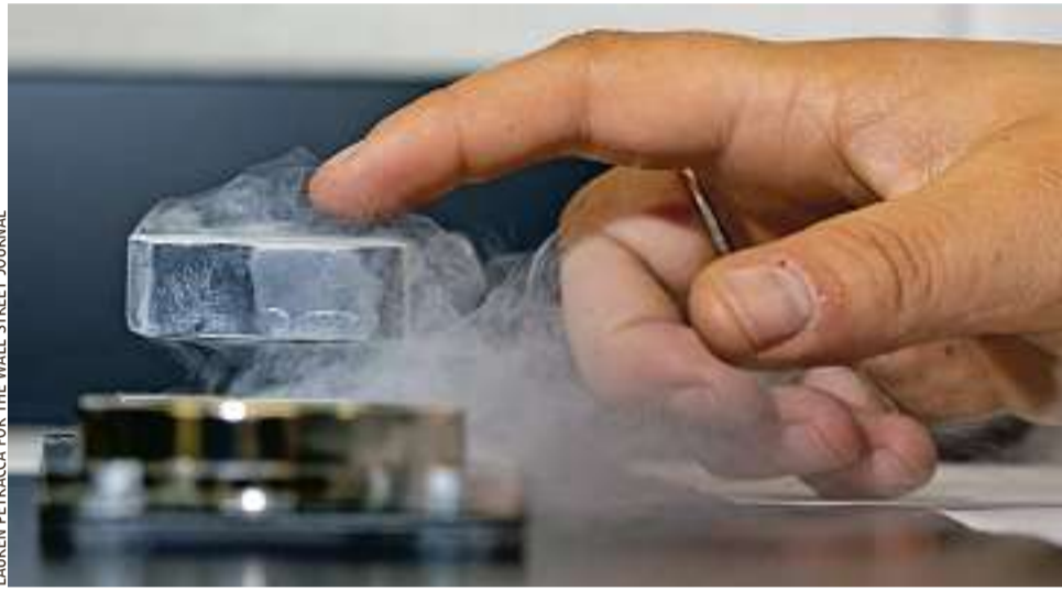
A superconductor at an extremely low temperature levitated above magnets at Rochester.
