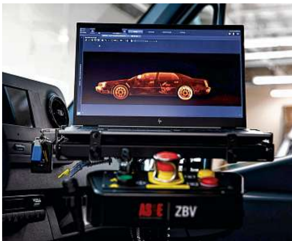
An image from X-ray scanning equipment in a van made by American Science & Engineering.
