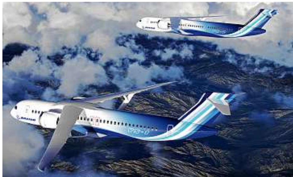
The prototype, to be built with NASA backing, would have longer, thinner wings for fuel efficiency.
