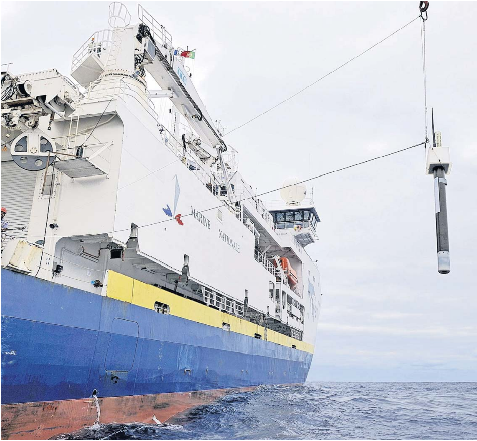
Data deep dive: deployment of a floating robotic observatory from a French research vessel in polar waters
