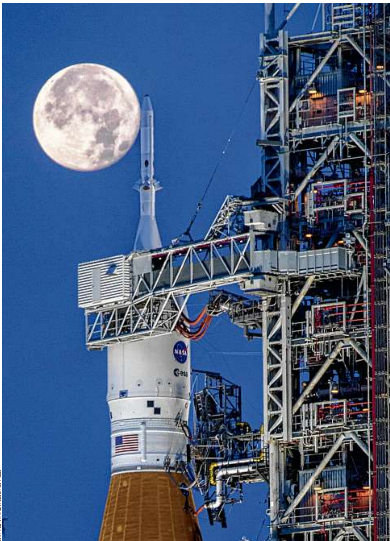
The Artemis I Space Launch System and Orion spacecraft, atop the mobile launcher, at NASA's Kennedy Space Center.
