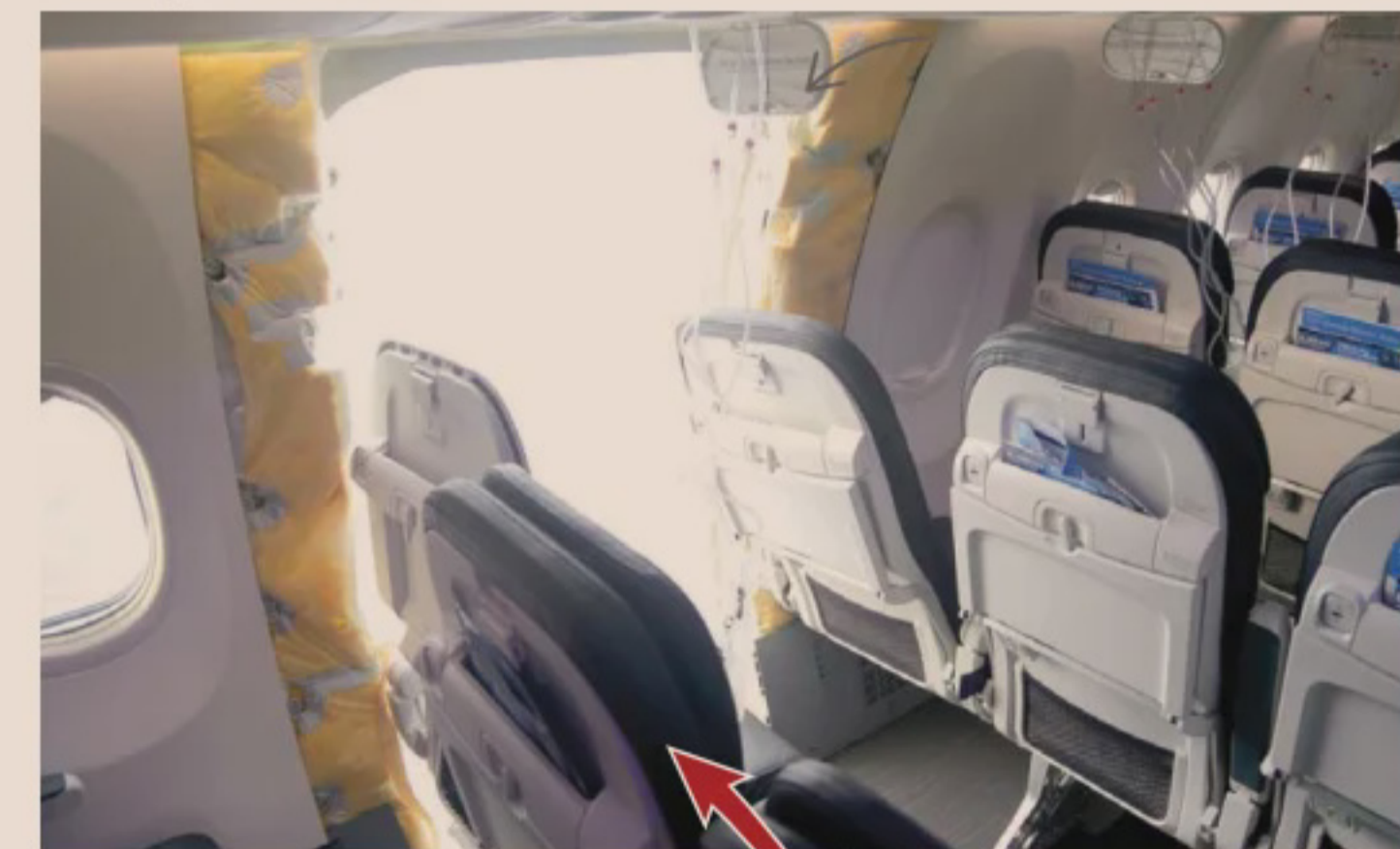
The area of fuselage that detached on Jan 6 comprised a mid-cabin door plug. This replaces an emergency exit door that is unnecessary when the aircraft layout has fewer seats
