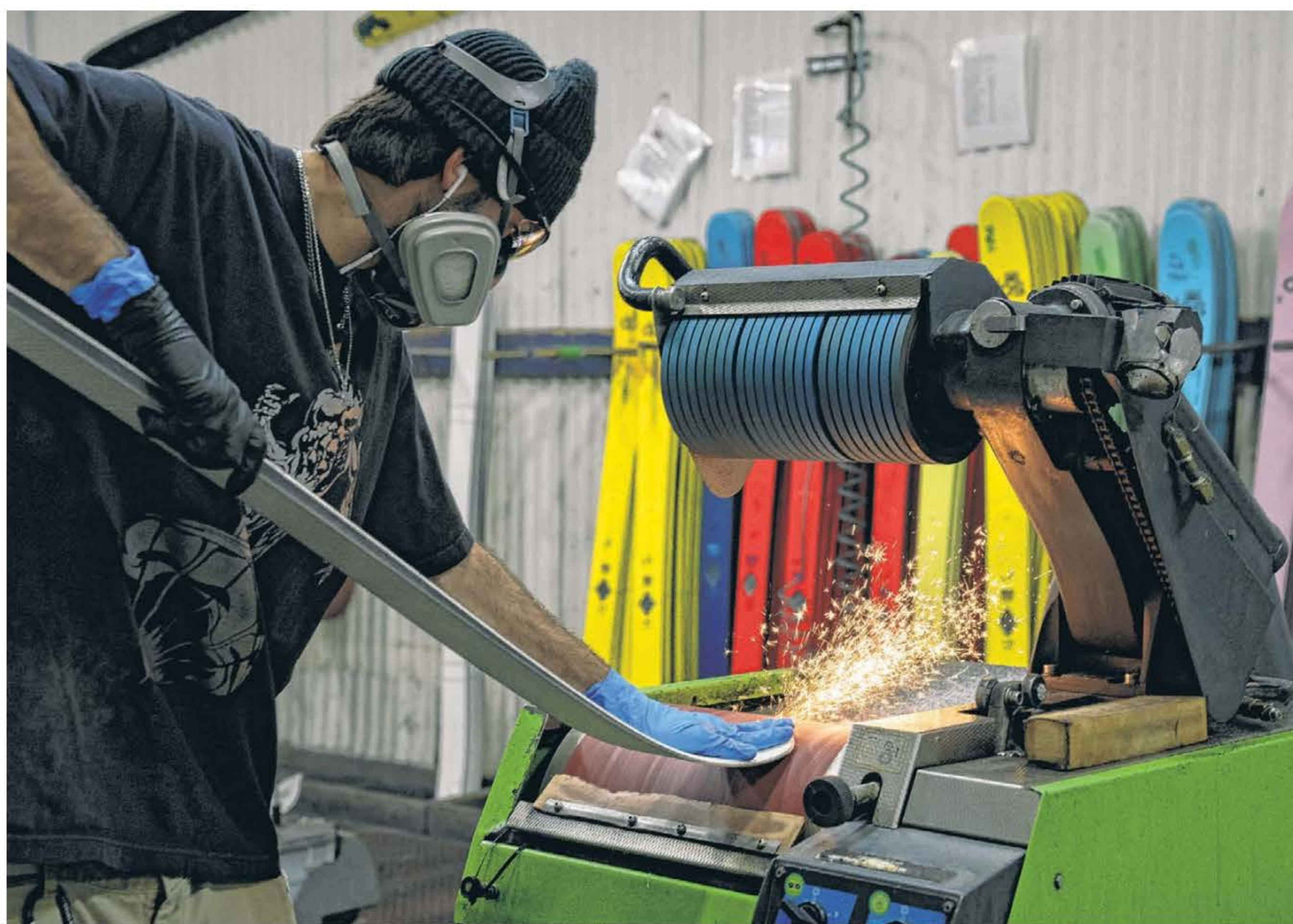
▲ A worker sands the bases of a ski at the DPS Skis factory in Salt Lake City.
