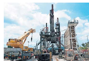
A drilling well at Enel's geothermal power plant site in Larderello, Italy
