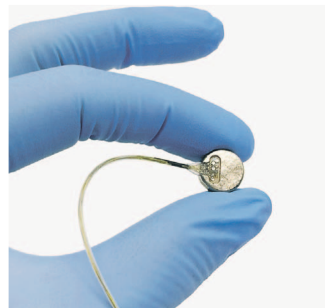
Paradromics's Connexus Cortical Modules target neurons just below the surface of the brain
