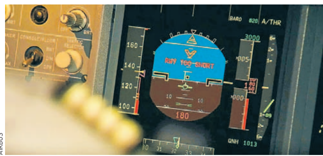
Airbus offers a runway overrun protection system on its jets.
