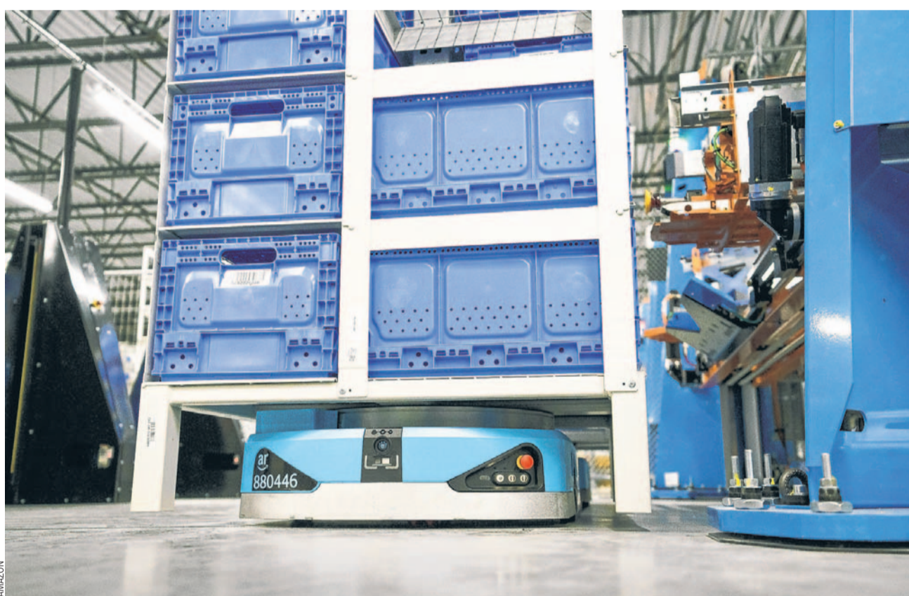
In the new Amazon robot structure, vehicles transport products inside tote containers to a new sortation machine.
